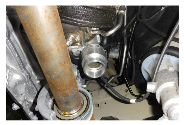
6. Using a 10mm socket and ratchet secure the supplied alloy hose joiner with the original fastener where the OE hard pipe mounted. Using a 7mm socket or flat blade screwdriver secure the OE rubber hose to the alloy hose joiner.
