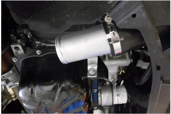
7. Fit silicone hose #2048 to the coupler and hose joiner as shown in the picture below. Using a 7mm socket and ratchet secure both ends of the silicone hose with the supplied hose clamps, 40-60 hose clamp is used for the coupler end of the hose. The 50-70 hose clamp is used for the hose joiner end of the hose.
