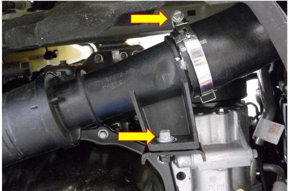
3. Using a flat blade screwdriver, lever the retaining clip away from the turbo to allow the coupler on the hose to release from the turbo. You will now be able to remove the hose from situ.
